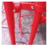
Picture shows height adjusting pins FULLY located and visible from the other side.
